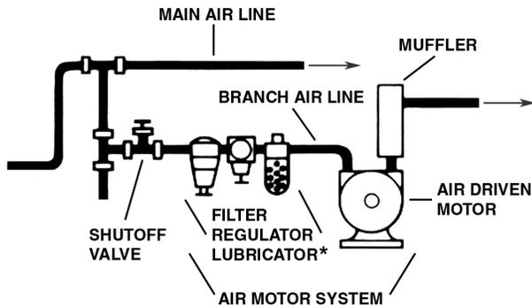
Check the direction of the motor airflow. A single rotation motor will operate properly only in one direction. Single rotation motors require a sound absorber to be connected to the air port. Remove the plastic shipping plugs from the ports. Save plugs for future use during shutdown.
